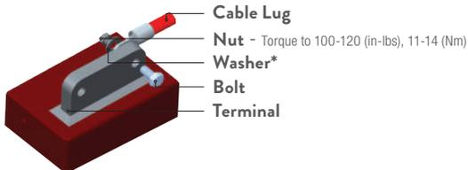
*Images shown reflect correct hardware placement. All hardware supplied for AGM with C-max and AES models, motive and solar.
